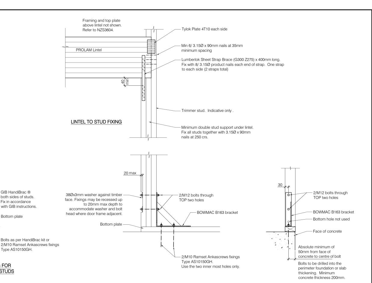
ALTERNATIVE BASE FIXING FOR FRAMING BOTH SIDES OF STUDS
